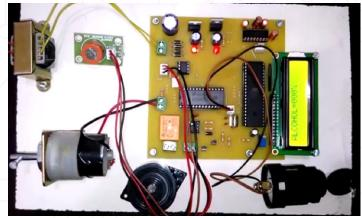
The purpose of this project is to develop vehicle accident prevention by method of alcohol detector in an effort to reduce traffic accident cases based on driving under the influence alcohol.
